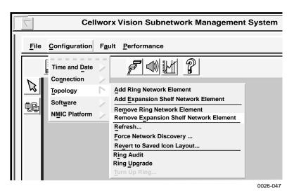
Figure 746-1. Remove EPS NE Pull-down Menu
